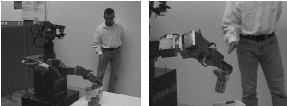
Figure 5: Interactive manipulator control: ARNOLD imitates the user's arm movement and grasps an object.
